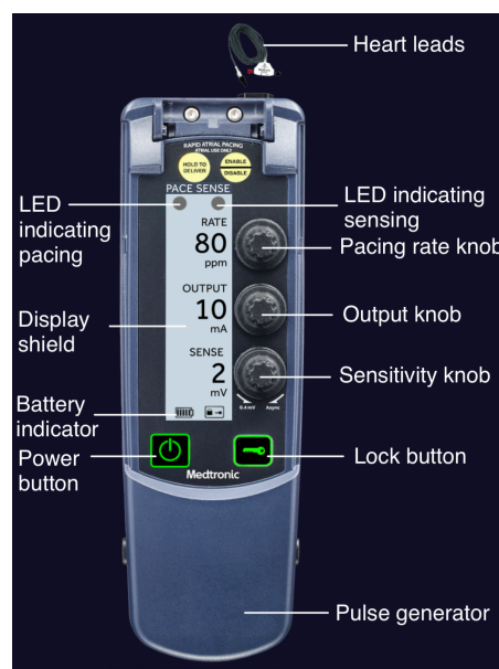
Figure 1: Components of Single Chamber Temporary External Pacemaker (Medtronic 53401) [8]
